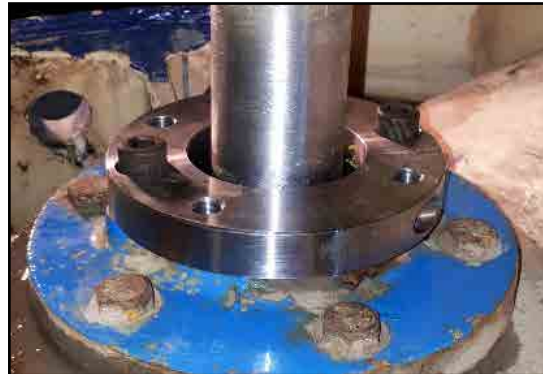
The 442 seal was adapted to fit the stuffing box.
